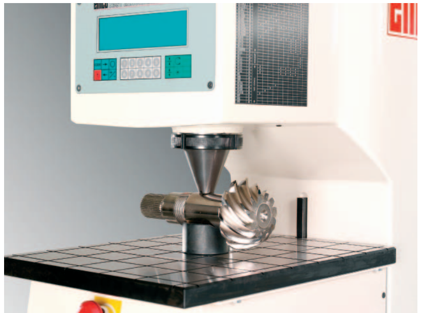
A suitable V-anvil takes up the part.
