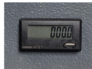
The hour counter registers the hours the cutting motor has been in operation
