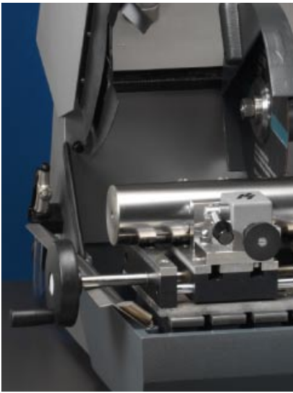
The adjustable cutting table enables parallel sectioning
