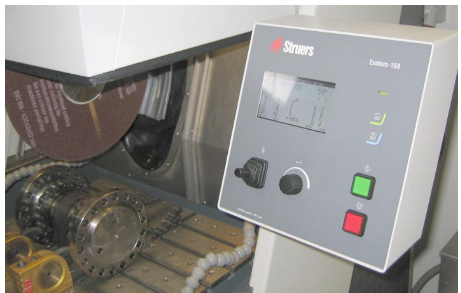
Two simple keys combined with a large graphic display are incorporated on a swivelling control panel
