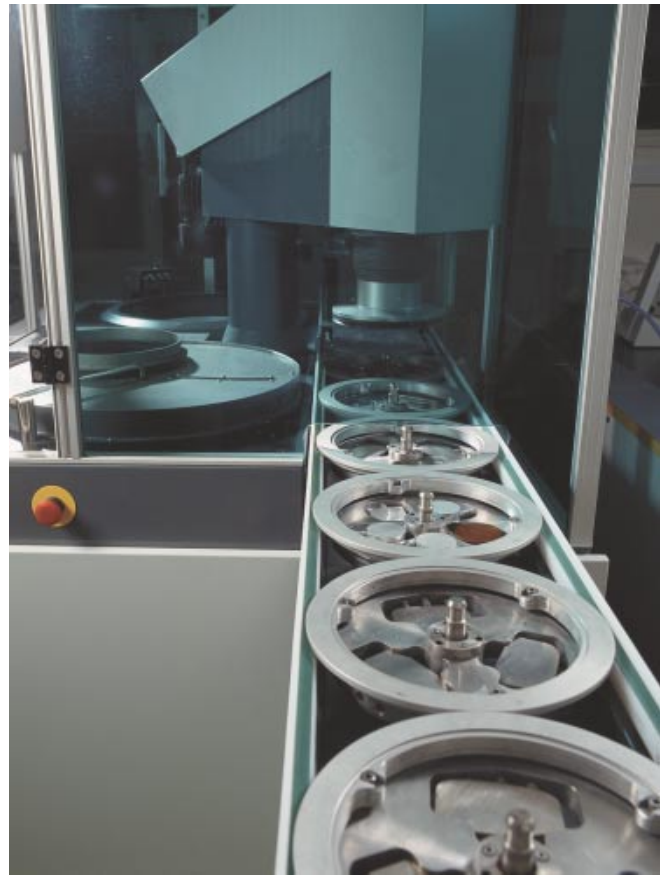
1. Six specimen holders queue up in the conveyer leading into MAPS
