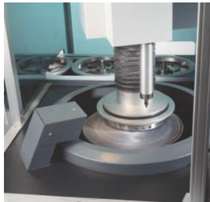
6. After fine grinding the specimen holder moves on to polishing
