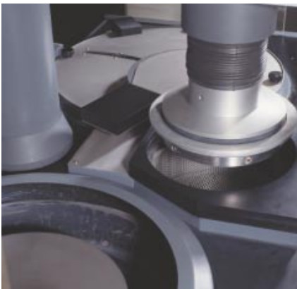
5. When the grinding is completed, the specimen holder is carried to the cleaning chamber
