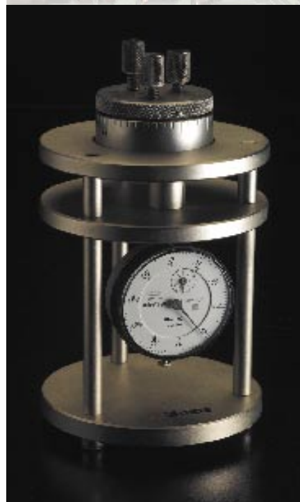
Multiple targets are aligned by placing AccuStop-T on the AccuMeter measuring station
