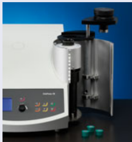
Easy access means quick change of mounting units and easy cleaning.
