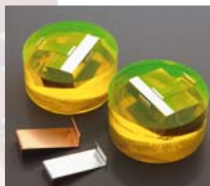
Taper section angles are available in steel, aluminium and copper. The angles make it much easier to measure the thickness of thin layers.
