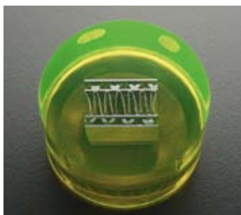
EpoDye, fluorescent dye for easy identification of all pores filled with mounting resin.
