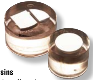
Polyesters are suitable for routine work and for quick mounting of specimens requiring low shrinkage and good wear resistance.
