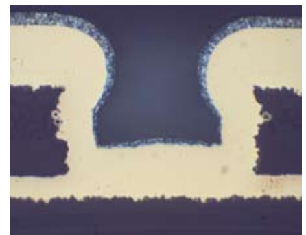
ViaFix can be used for microvias down to 100 µm. Blind microvia unetched, x500.
