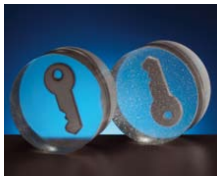
ClaroCit mounts cured with pressure (left) and without pressure (right).
