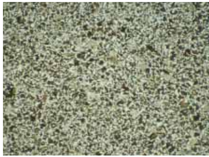
Pure copper. Sample etched with cupric chloride and ammonia. Magnification x100
