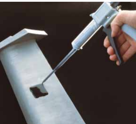
An operator dispenses RepliSet onto a sample
