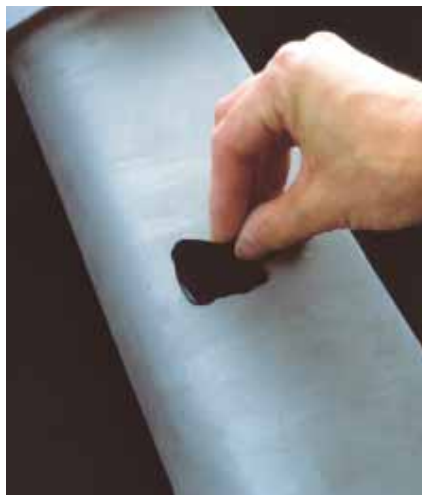
An operator peels off the cured replica
